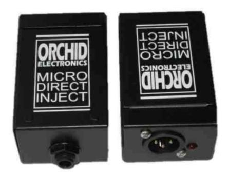
Housed in a strong sheet steel case 80 X 50 X 40 - it has only a jack socket input for connection to the instrument and an XLR output to feed the microphone input of a mixing desk - which can be located many hundreds of metres away if necessary. It must receive Phantom Power from the mixer as it is an active design - a red LED will indicate power present.
